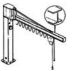
H Series - "H" overbraced jib model Capacity 250 to 2000 kg - Jib length 4 to 8 m
